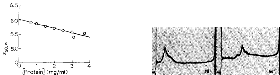
Fig. 4. Concentration dependence of sedimentation coefficient of plasmodium myosin A. Solvent conditions: 0.5 M KCl, 10 mM Tris-maleate buffer (pH 7.0). Ultracentrifugation was carried out at 59780 rev./min at 11.2°.
